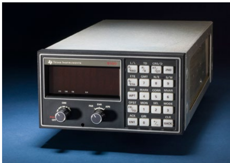
A LORAN-C receiver, circa 1980, is only one of the old tools we’re not using anymore. LORAN-C offered mariners better precision than its predecessors, but it was still imprecise beyond half a mile. (Photo: Dane Penland, Smithsonian National Air and Space Museum - NASM 2012-02114)
